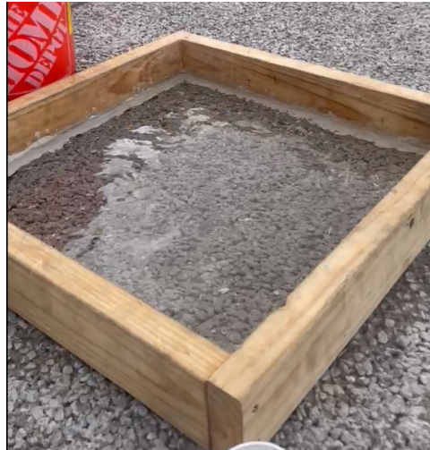
Figure 16: Simple infiltration test apparatus
