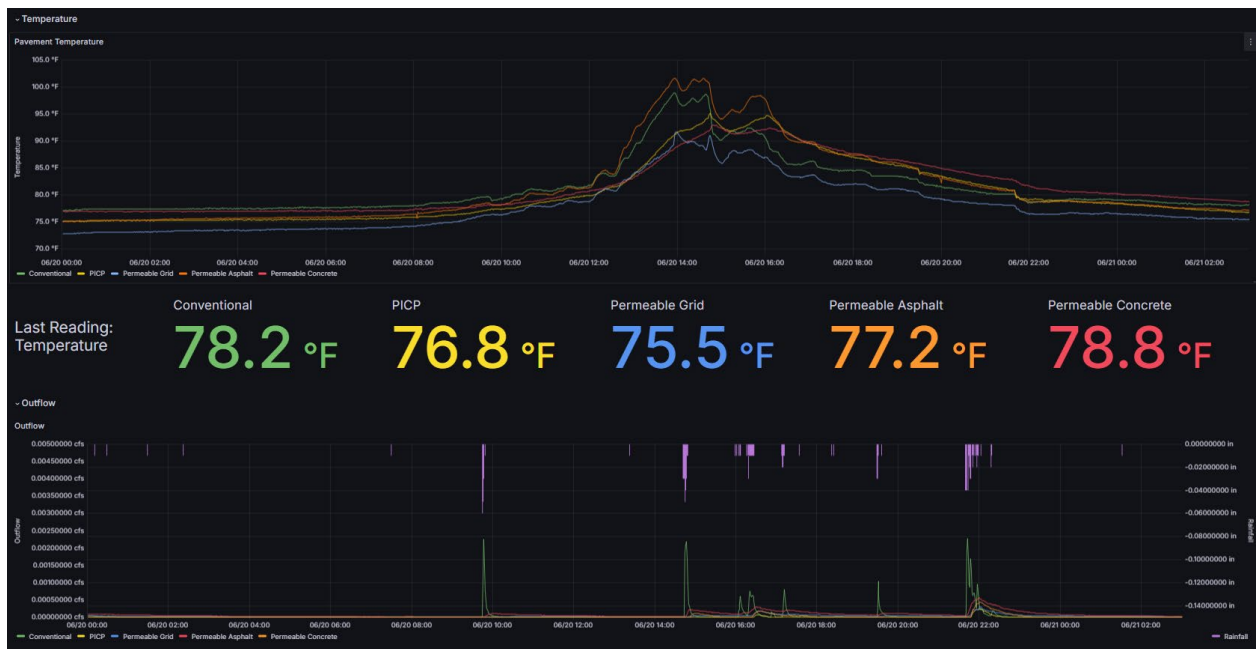
Figure 15: RTM Dashboard: Pavement temperatures are displayed at the top, with real-time hydrograph and precipitation data at the bottom streamlined in real-time after an event
