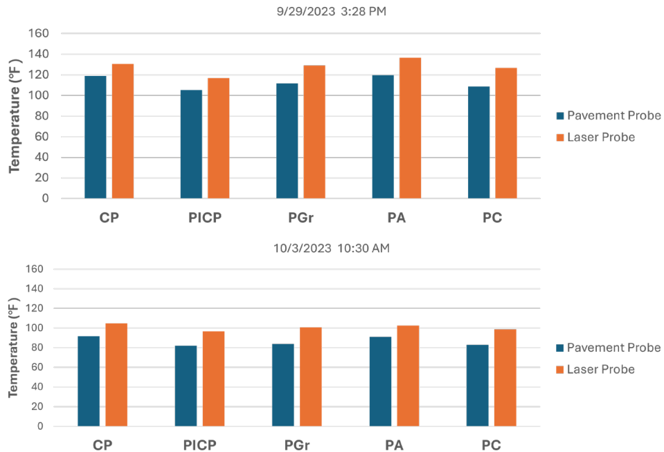
Figure 45: Temperature differences between pavement surface and permeable layer bottom
