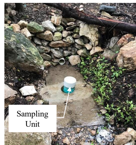
Figure 12: Basin Outlet Sampling Point for Stormwater
