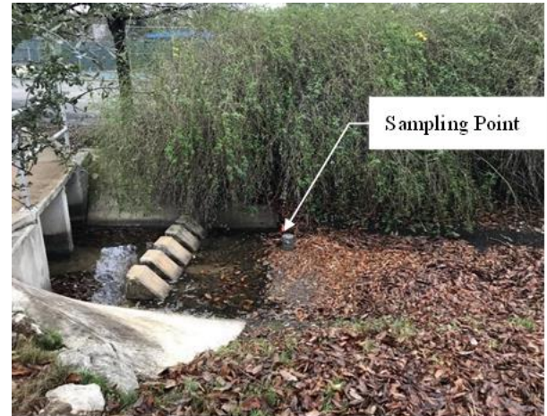
Figure 11: Inlet Sampling Point for Pre-Construction Soil and Stormwater and Post-Construction Stormwater
