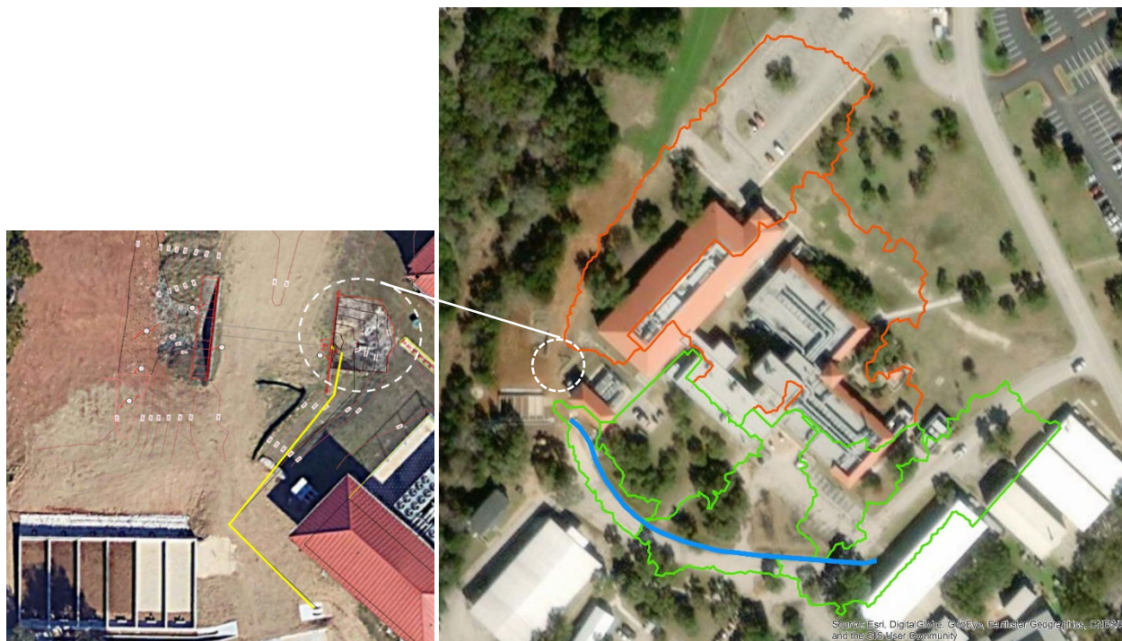
Figure 3- 10. Pump system installed in November 2020 to expand the contributing drainage area
